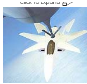
To accommodate in-flight refueling, a low observability in-flight refueling receptacle is integral to the aircraft dorsal spine.
