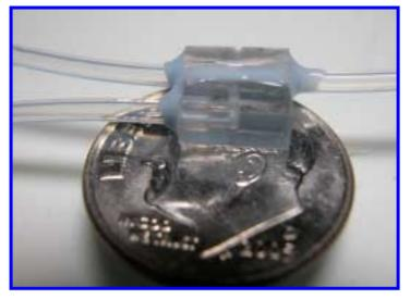
Pneumatically controlled vacuum valve used to isolate vacuum system from atmosphere to a lower pressure limit of 10-4 torr.
