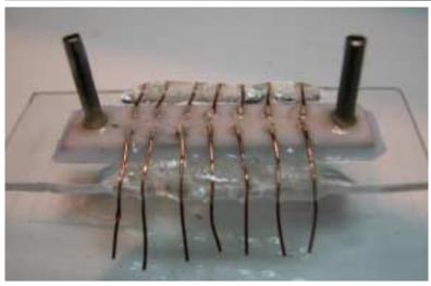
Reverse side of above experiment showing both cathode gas inlet line and anode vacuum line. Leads are temporarily attached to metal terminals with conductive cement. Entire experiment can be lifted off glass cover plate then modified and replaced without harming the elastomer seal.
