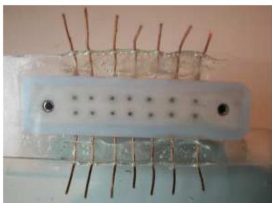
Ceramic EVO experiment with EVO source on right and anode on left with 14 leads brought out of the active region for whatever purpose is needed. Device is about 1 inch long.
