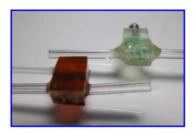
Pneumatically operated valve and controlled leak used to set gas pressure in various regions of experiments. The valves are 0.2 inches long with 1/16-inch diameter connection tubes.
